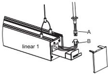
Disconnect the A and B parts.
