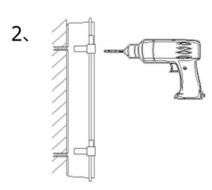
Put the fixture on the wall,drill 3 holes to get through the housing
