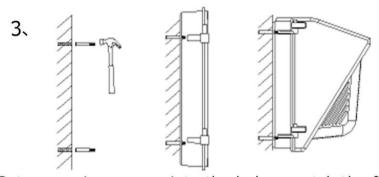
3. Get expansion screws into the holes, match the fixture to the bolts, then fix the fixture on the wall by screws, lastly get the PC cover and fixture housing back together
