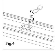
3-Turn off the power,make the wire connection to the quick connector
