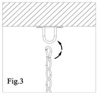
2-Hook up the chain on the ceiling anchor
