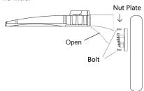
**Step 2:** Connect the AC wire of the fixture and tighten the water-proof gasket and cover plate on the arm by screws,then power on.
