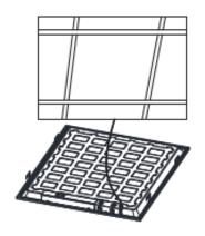
③ Fix the panel light into plaster ceiling.
