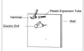
3 Use the electric drill to punch the hole at the mark position Ø8mm, depth 40mm; and use a hammer to drive the plastic expansion tube into the hole;
