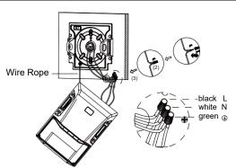
4. Fix the bracket with a screwdriver, and fix the fixture installation wire rope on the mounting plate, connect the cable as shown and do a good waterproof treatment;
