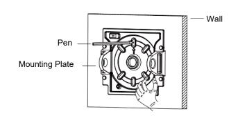
After knocking out the mounting holes with a hammer (at least 2 mounting holes and they should be in a symmetrical position), press the bracket on the wall with your hand and mark with the pen at the mounting screw position;
