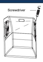
1. Disassemble the fixing screws of the lamp mounting plate with a screwdriver and remove the mounting plate;
